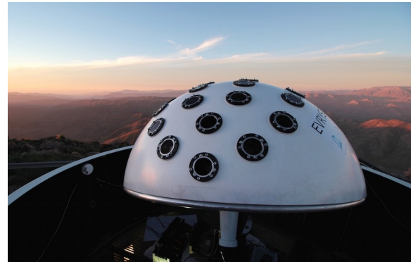
The Southern Evryscope deployed in the Chilean Andes. The system is a 23-telescope array mounted into a hemisphere which tracks the sky.
